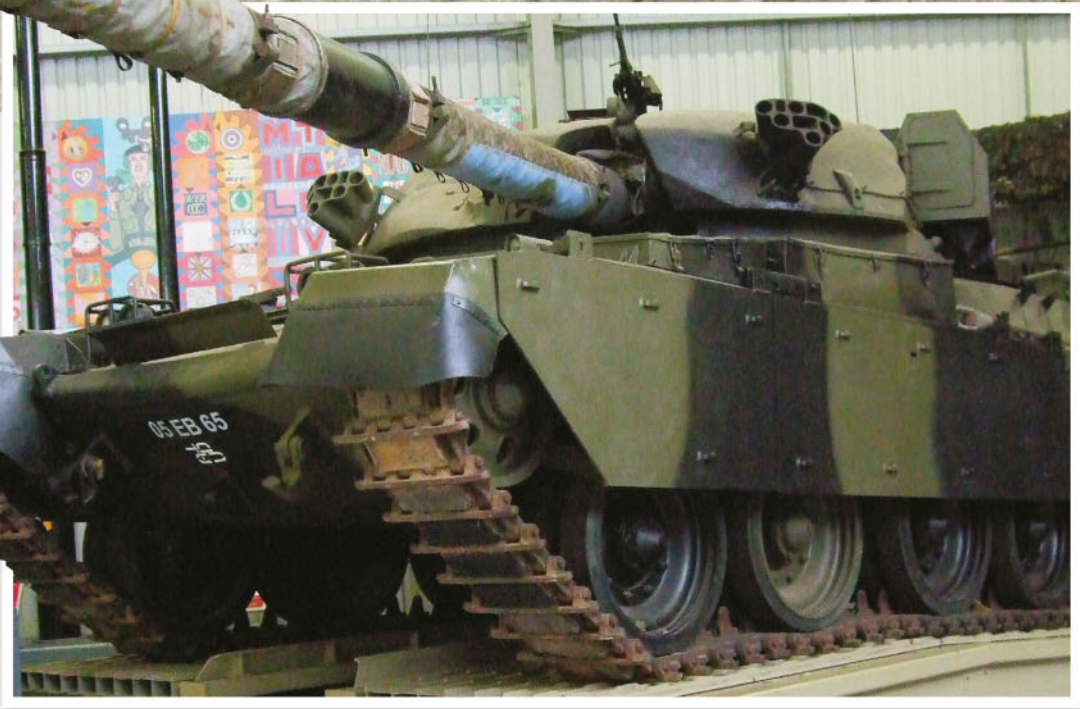
Right: Secondary smoke grenade launchers are visible on either side of the turret. Note the cupola-mounted 7.62mm L37A1 machine gun
